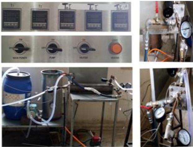
Figure 3: Experimental Setup of Floating Head Multi Stream Heat Exchanger
