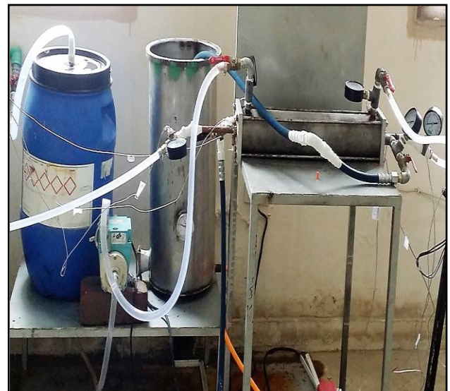
Figure 2: Floating Head Multi Stream Heat Exchanger
