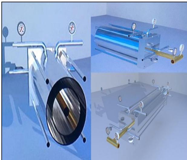
Figure 1: Internal View of Floating Head Multi Stream Heat Exchanger
