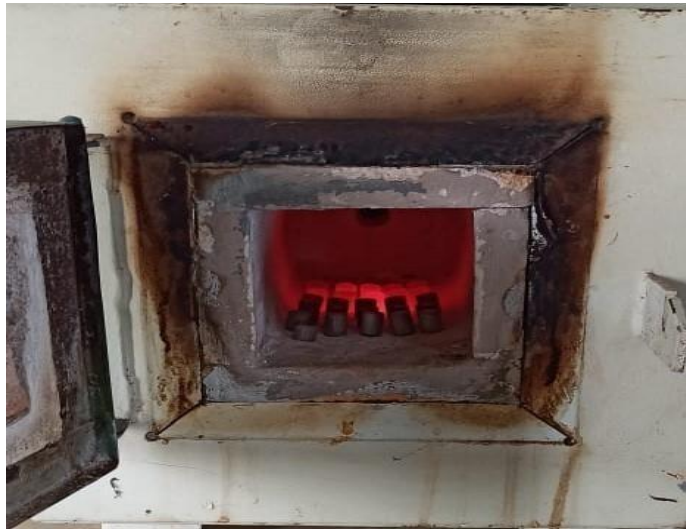
Fig. 7INSIDE VIEW OF MUFFLEFURNACE
