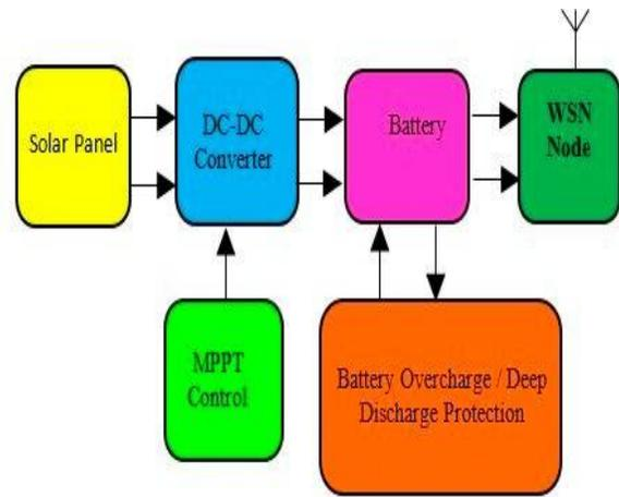
Fig4. Block diagram of solar energy harvesting system using MPPT control.
