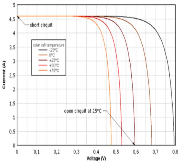
**Fig. 11: I-V curve at various temperature and constant irradiance**
