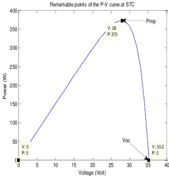
Fig. 6: P-V curve adjusted to three remarkable points at STC
