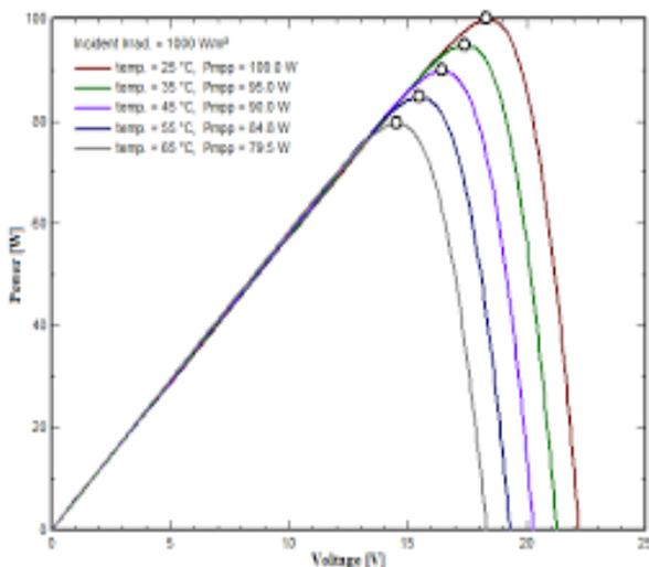
**Fig. 12: P-V curve at various temperature and constant irradiance**
