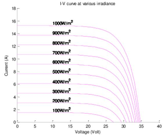
Fig. 8: I-V curve at various irradiance and constant temperature
