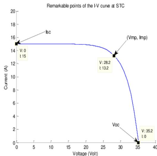
Fig. 5: I-V curve adjusted to three remarkable points at STC
