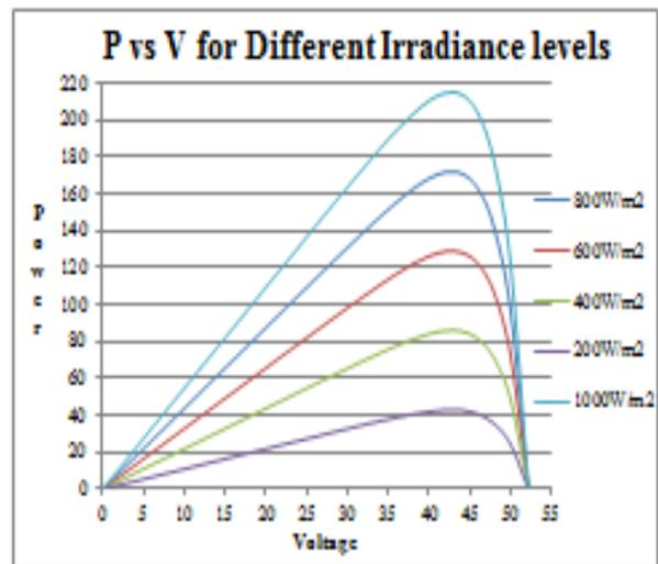
Fig. 9: P-V curve at various irradiance and constant temperature
