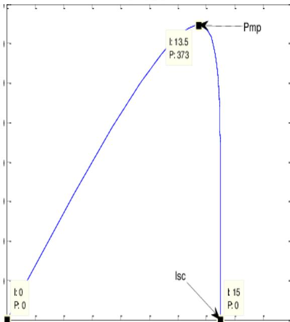
Fig 7 P-I curve adjusted to three remarkable points at STC
