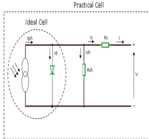
**Fig 2. General model of PV cell in a single diode model**
