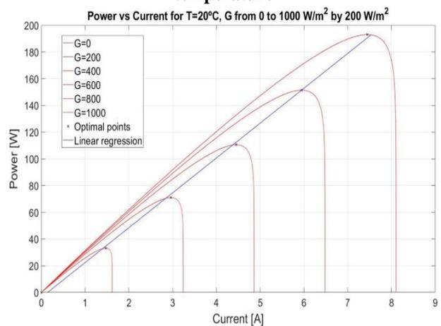
Fig. 10 : P-I curve at various irradiance and constant temperature
