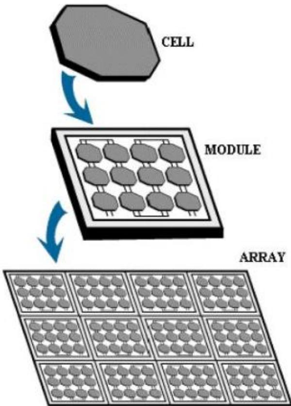
**Fig1. Photovoltaic Hierarchy**
