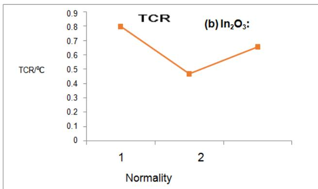
**Figure 3.6** TCR graph of binary oxide In<sub>2</sub>O<sub>3</sub>: MoO<sub>3</sub> thin film with concentration 0.2N:0.1N
