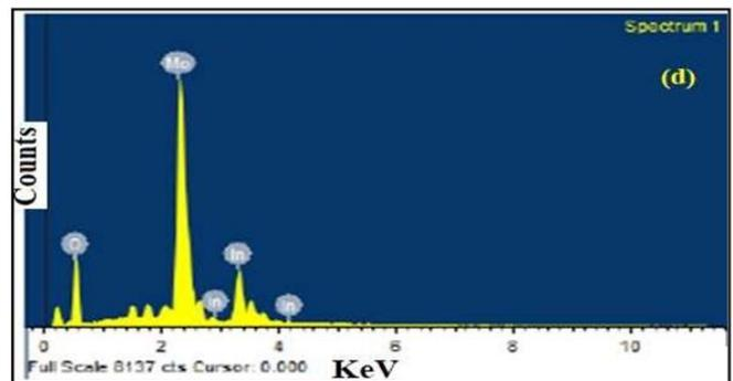
Figure 3.3 EDS of Binary oxide In<sub>2</sub>O<sub>3</sub>: MoO<sub>3</sub> thin film with concentration 0.2N:0.1N
