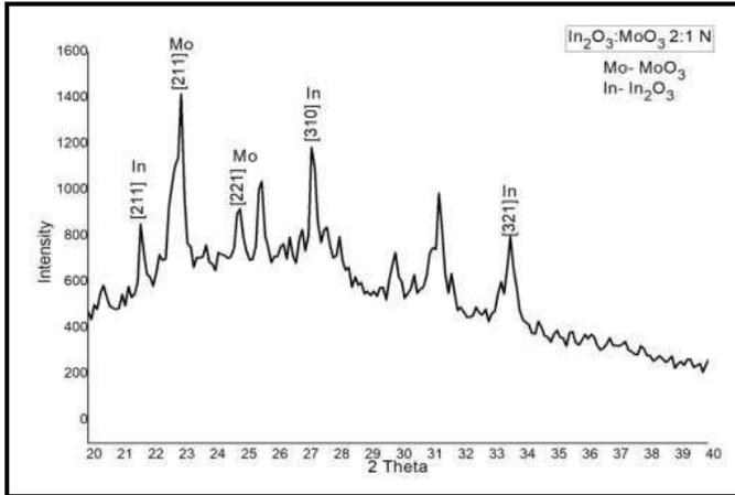
Figure 3.1 XRD of Binary oxide In<sub>2</sub>O<sub>3</sub>: MoO<sub>3</sub> thin film with concentration 0.2N:0.1N
