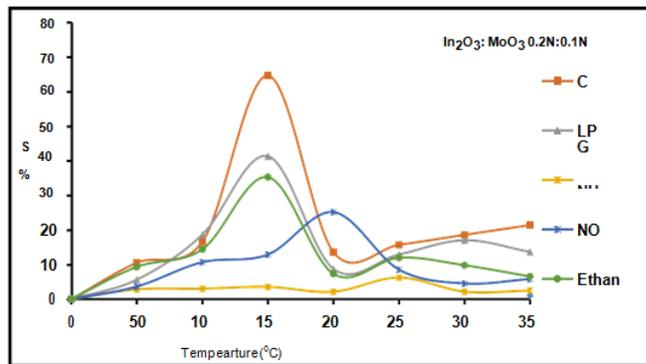
**Figure 3.7** Gas sensitivity response of Binary oxide In<sub>2</sub>O<sub>3</sub>: MoO<sub>3</sub> thin film with concentration 0.2N:0.1N
