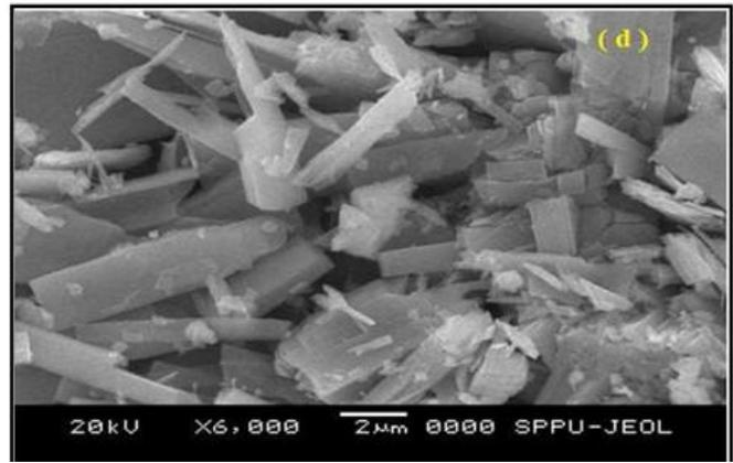
Figure 3.2 SEM of Binary oxide In<sub>2</sub>O<sub>3</sub>: MoO<sub>3</sub> thin with concentration 0.2N:0.1N
