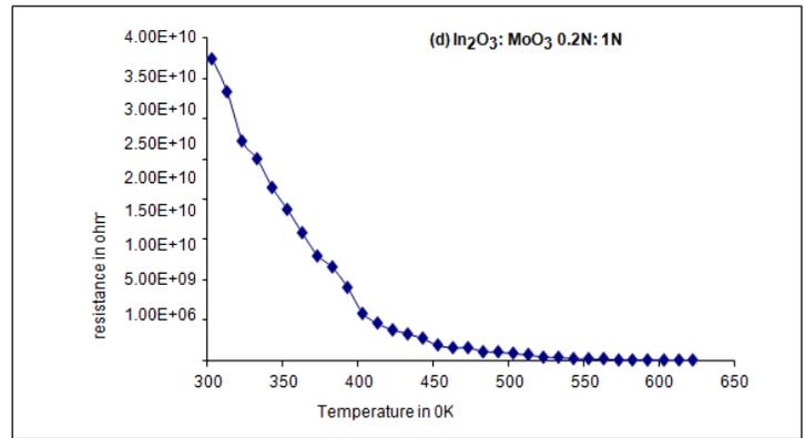
**Figure 3.4** Resistance of Binary oxide In<sub>2</sub>O<sub>3</sub>: MoO<sub>3</sub> thin film with concentration 0.2N:0.1N
