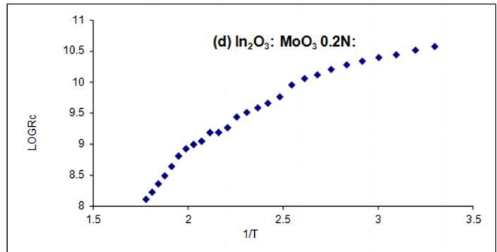
**Figure 3.5** Activation energy of Binary oxide In<sub>2</sub>O<sub>3</sub>:MoO<sub>3</sub> thin film with concentration 0.2N:0.1N
