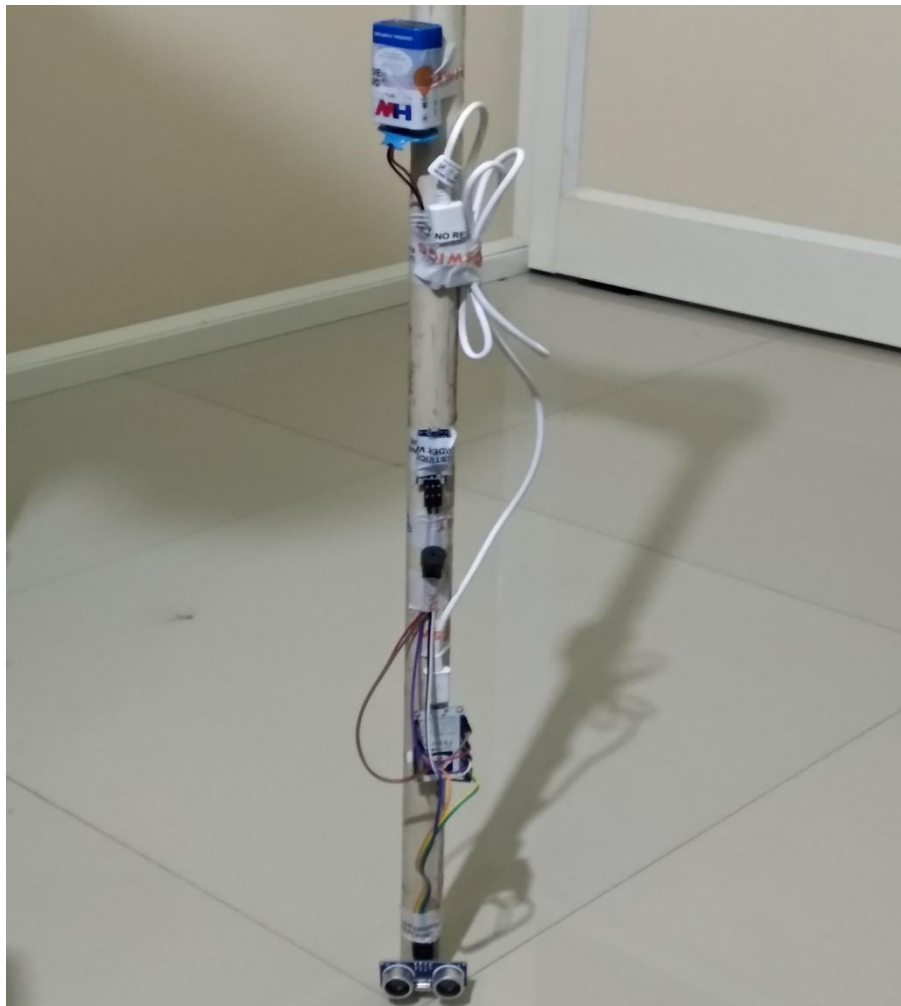
Figure 2: Ultrasonic Blind Walking Stick
