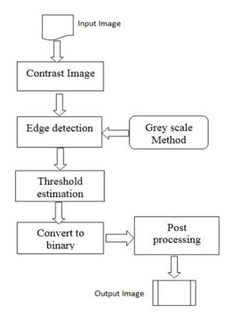
The proposed system proposes document image binarization techniques. Given a degraded document image, an adaptive contrast map is first constructed and the text stroke edges are then detected through the combination of the binarized adaptive contrast map and the canny edge map. The text is then segmented based on the local threshold that is estimated from the detected text stroke edge pixels. Some post-processing is further applied to improve the document binarization quality.
