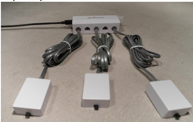
Figure 1 Wired Sensor Connection
