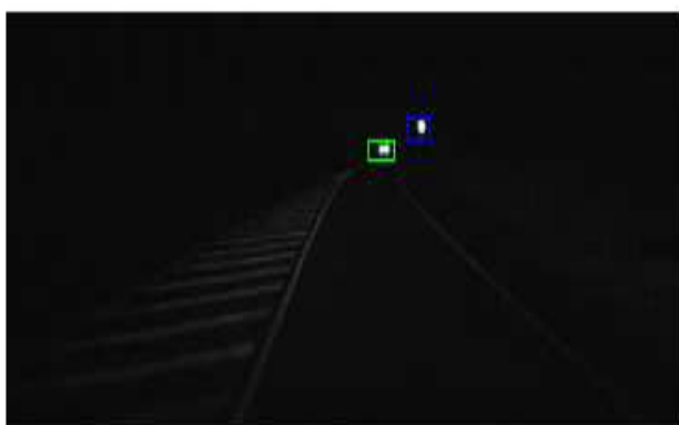
Figure 2 Detection of headlights at 70 m [1]
