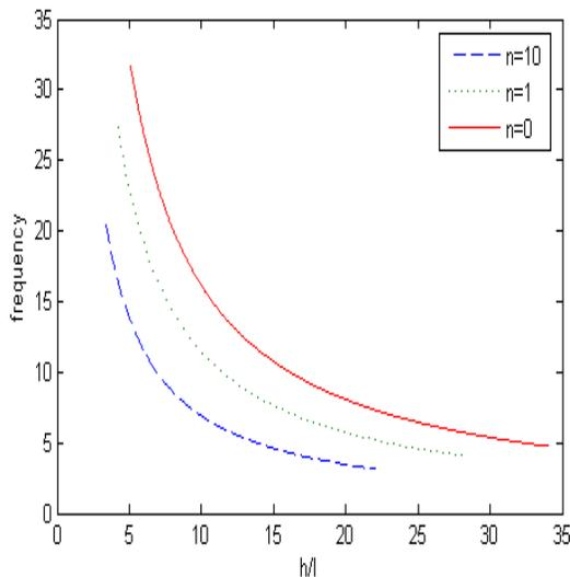
**Figure 11. Effect of length scale parameter on Nano rectangular FG plate frequency**
