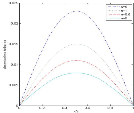
Figure 6. Dimensionless deflection of Nano rectangular FG plate with constant length scale parameter ( $h/l=1$ ) and different power law index
