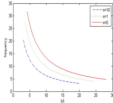
**Figure 13. Effect of length scale parameter on Nano rectangular FG plate frequency**
