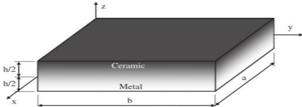
Figure 1: Geometry of FGM plate[17]
