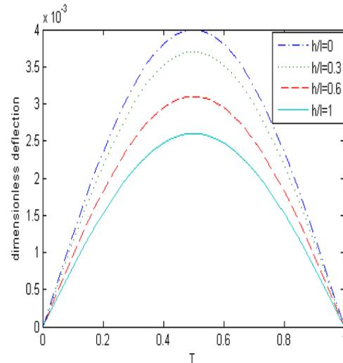
Figure 8. Dimensionless deflection with constant power law index ( $n=1$ ) and different length scale parameters under moving load throughout of time
