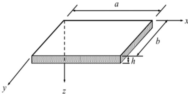
Figure 2. The geometry of a Nano rectangular FG plate[25]
