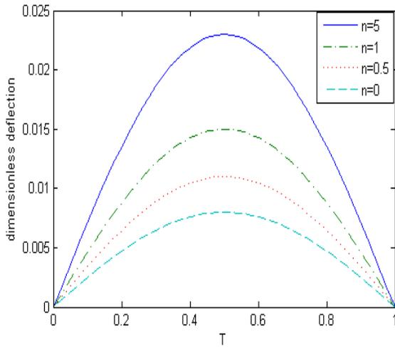
**Figure 10. Dimensionless deflection with different power law index and constant length scale parameter ( $h/l=1$ ) under moving load throughout of the time**
