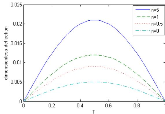
Figure 7. Dimensionless deflection with different power law index and constant length scale parameter ( $h/l=1$ ) under moving load throughout of the time
