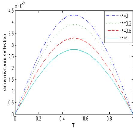
**Figure 9. Dimensionless deflection with constant power law index ( $n=1$ ) and different length scale parameter under moving load throughout of the time**
