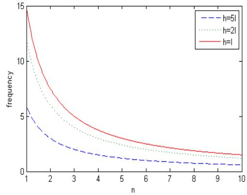
**Figure 12. Effect of power law index on Nano rectangular FG plate frequency**
