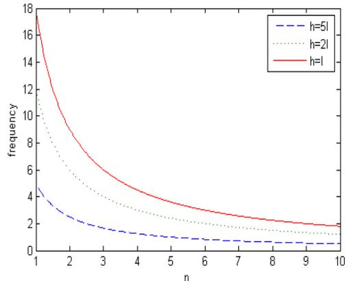
**Figure 14. Effect of power law index on Nano rectangular FG plate frequency**
