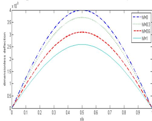
Figure 4. Dimensionless deflection of nano rectangular fg plate with constant power law index ( $n=1$ ) and different length scale parameter at  $x_0=x$  and  $y_0=b/2$
