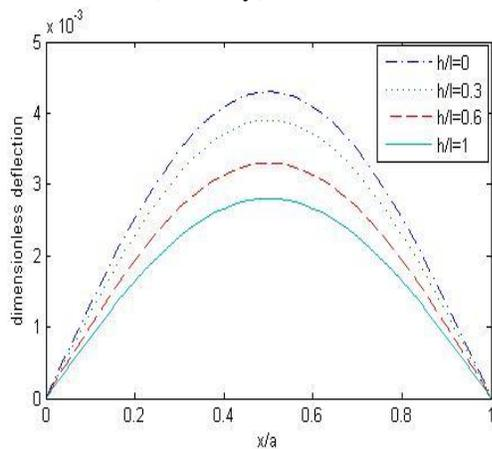
Figure 5. Dimensionless deflection of Nano rectangular FG plate with various length scale parameter and constant power law index ( $n=1$ ) at  $x_0=x, y_0 = \frac{b}{2}$
