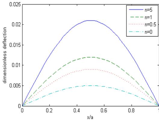
Figure 3. Dimensionless deflection of nano rectangular fg plate with different power law index and constant length scale parameter ( $h/l=1$ ) at  $x_0=x$  and  $y_0=b/2$
