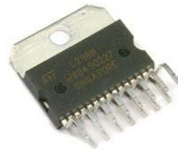
Figure 6: Motor Driver IC L298 [7]
