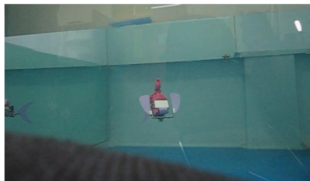
Under Water Swimming Test Fin type Fish robot
