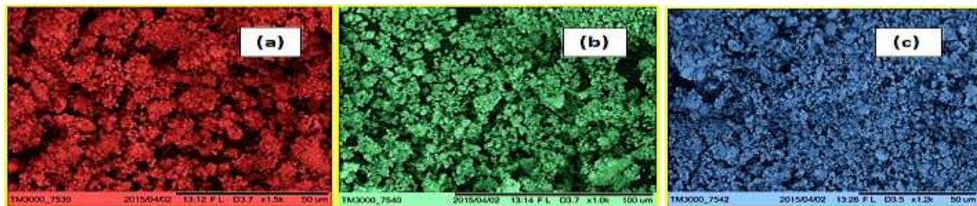
Figure 4 : SEM images of ZnO (a) 2ml (b) 4ml and (c) 6ml latex.
