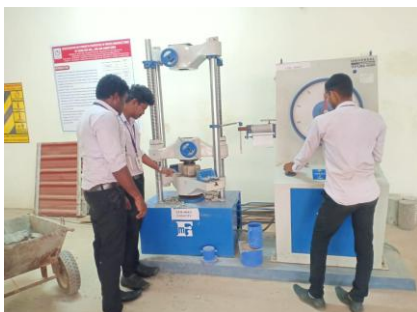
Figure 2. Compressive strength testing of a paver-block specimen.
