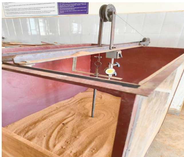
Figure 3. Laboratory pull-out test tank and loading arrangement.
