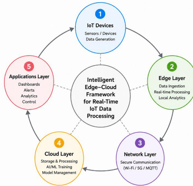
Fig 1. Circular Architecture of an Intelligent Edge-Cloud Computing Framework for Real-Time IoT Data Processing.
