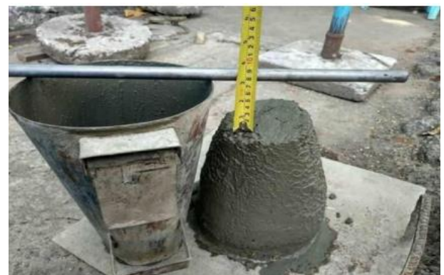
Workability values for different concrete mix M-20
