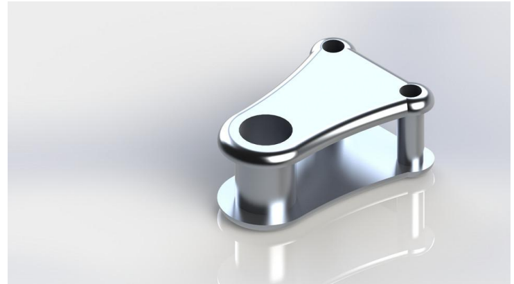
Fig. 2: Optimized Pitman Arm Geometry (Slot Design)
