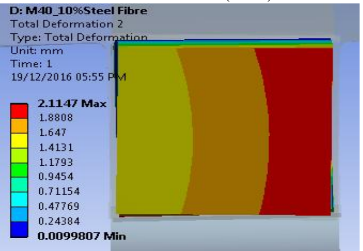
Fig.5.23. : Snapshot of twisted shape of R.C. beam model for M40 grade model (10% steel fiber)
