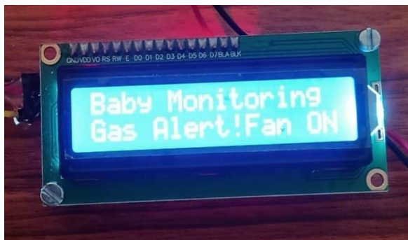
Fig-9: Output of Methane Sensor
