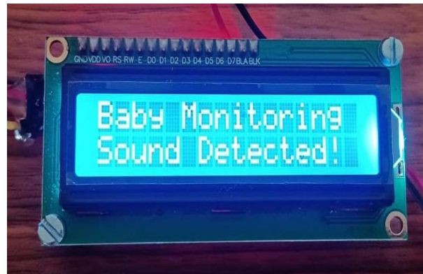
Fig-7: Output of Sound Sensor
