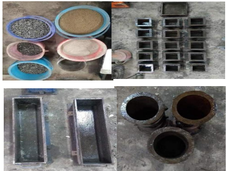
Figure 5.1 Prepared material, Moulds ,Beams and Cylinder
