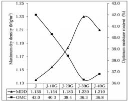
This behavior is attributed to the particle packing phenomenon, where GGBS particles fill the voids in jarosite, leading to denser packing and higher dry density up to an optimal point. Beyond this, excess GGBS causes segregation and weak bonding, reducing MDD.
